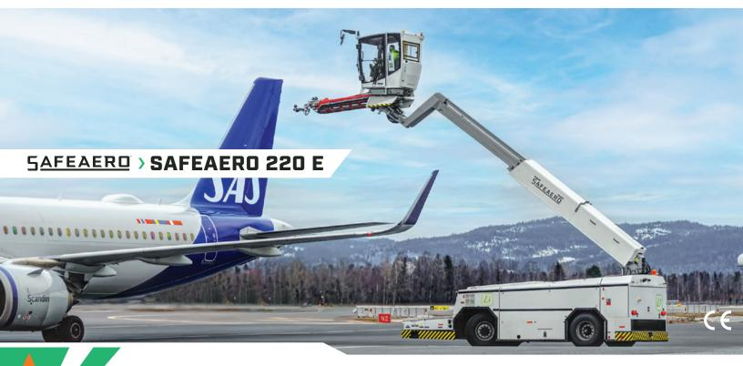
Powered by lithium batteries, The Safeaero 220 E with Intellimix™ technology increases productivity and decreases environmental impact through eliminating the need to purge fluids between planes.
